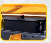
Oil tank for automatic chain lubrication with an oil level indicator.
