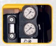
The pressure gauges indicate the splitting pressure and the system pressure for auxiliary functions.
