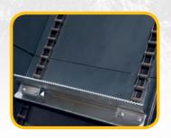
Logs are transported by the conveyor belt with a bar-link chain.
