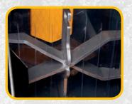
Electro-hydraulic height adjustment of the splitting knife 2-4, 2-6, 2-8, 2-12.
