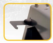
Shutter for retaining the log deck during transport.
