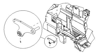
Lubricate knife adjustment at grease nipple indicated
