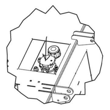
Replace the Filter cartridge (2251065) in the oil filter (1) after the first 50 operating hours and afterwards once a year of after 500 operating hours (depending on whatever occurs first)
