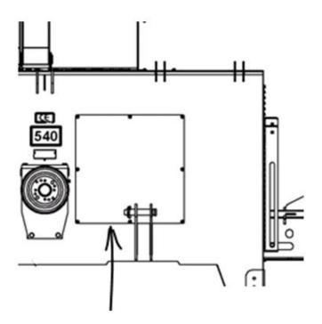
Open lid covering oil tank and clean the area to avoid that the oil tank is covered by dust and chips. This in order to keep up a best possible cooling effect.
