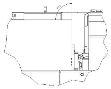
Inspect cutting chain and saw bar regularly. Sharpening ang tightening of the saw chain ensure effective cutting. Check that the vertical angle of the saw bar (90 degrees) so that the saw bar does not jam during cutting.
