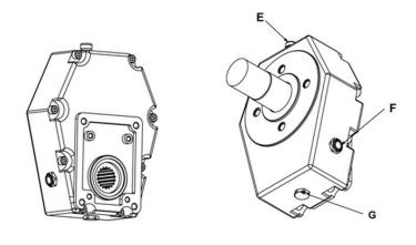
Check the oil level after each season by releasing level screw F as illustrated in the sketch (the oil to leak at sufficient level). Topping up via the breathing plug E on the top of the drainage via the plug G.
