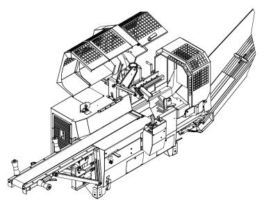
The covers over the chain bar and the cover over the splitting cradle can be opened as illustrated
