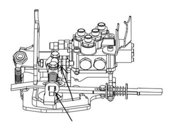
Grease the splitting mechanism lightly at indicated points in order to ensure smooth operation and reduce of wear.
