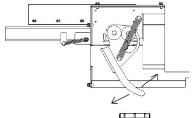
Clean the mechanism for the log stop function. Check that indicAted lever can move completely to the lower position
