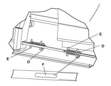
The stop signal and the return signal for the splitter piston are produced by contact with the spring loaded discs E. This point of contact may be adjusted by placing the screw D in the groove F.
