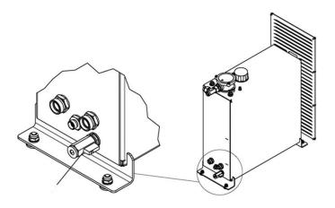
Drain a small amount of hydraulic oil to check the oil regularly. Grey oil is an indication of water in the oil. If this occurs, all hydraulic oil must be replaced.
