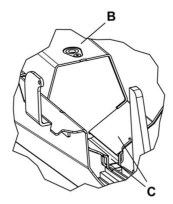
Bearing points for the splitter cylinder should be lubricated frequently during operation. The lubrication point for this is nipple B. Gliding surfaces in the groove for the splitter piston + other gliding surfaces should be lubricated when needed.
