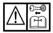
Before any sharpening work is initiated – stop the machine and tractor and remove the key to ensure unintentional start during the work.
