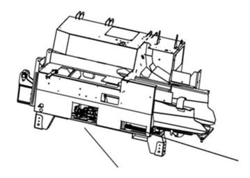
Open lids in front to the left and right as indicated and clean mechanism for eventual contaminations.
