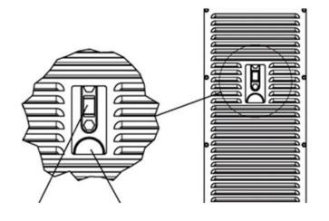
Check oil level and temperature of hydraulic oil regularly.
