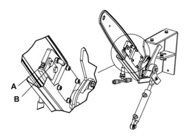
To replace the chain, the screw A is released (first release the nuts B) as far so at to allow the chain to be removed in the back for maintenance or replacement.
